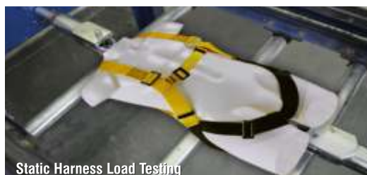
Static Harness Load Testing
