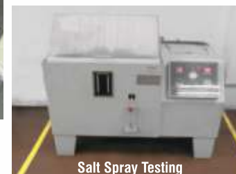
Salt Spray Testing
